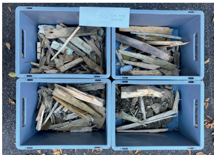
The range of fuels being tested: Biofuel mixes that are being analyzed at KIT with regard to their potential for generating deposits. (Photo: Kolb / KIT)
